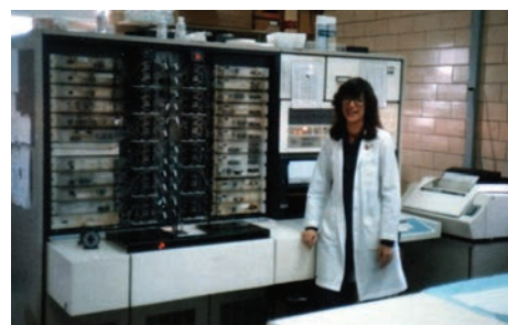
By the 1970s, clinical lab testing had moved well beyond individual manual procedures. This 1982 photo shows Clinical Lab Scientist Donna Frick in front of a SMAC (Simultaneous Multi-Channel Analyzer and Computer) at the Bryn Mawr Hospital lab. The SMAC could efficiently perform 20 different blood chemistry tests from a single patient specimen.
